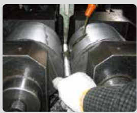
전조로링 (CYLINDRICAL THREAD ROLLING)
